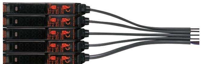
The **E3X-DA-S** requires three wires for the master sensor only. Each additional sensor in a group requires only one wiring connection. **Shown: ONLY 7 WIRES** with no additional extension connectors.
